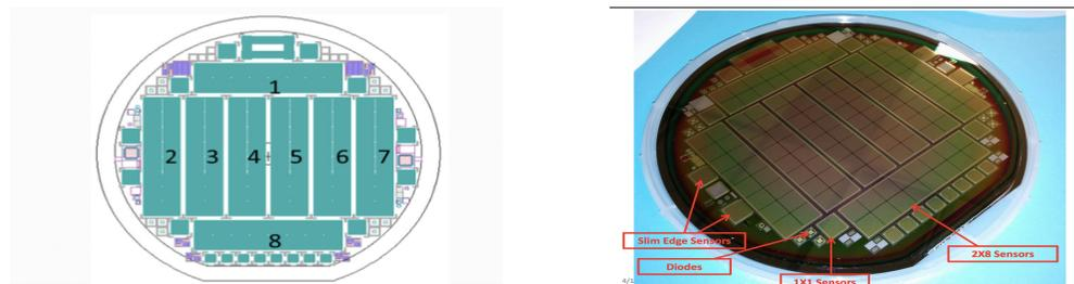
**Figure 6.5:** Sintef 2x8 sensor numbering (on the left). A picture of a wafer (on the right).
