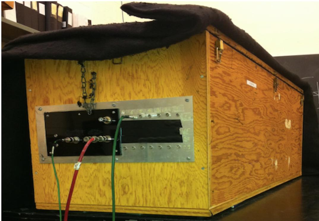
**Figure 7.1:** Light-tight box located at the University of Iowa PMT test station.
