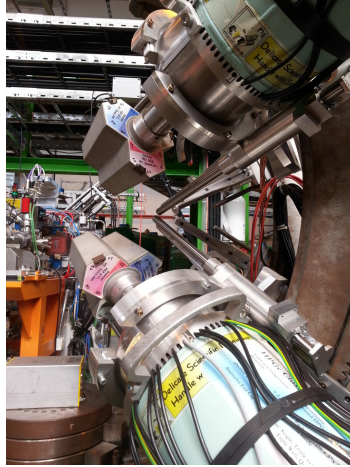
Figure 4.6.: Photograph of two MINIBALL triple clusters mounted on their frame at the MINIBALL experimental site. Looking upstream, with perpendicular offset to the beam line.
