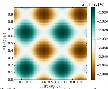
Figure 6: Visible cross-section bias as a function of phase advances between two collision points, for the typical vdM beam parameters, as obtained analytically.
