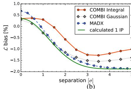
Figure 5: BB bias on the luminosity as a function of separation as calculated using the Gaussian distribution-based luminosity formula compared to COMBI and MADX simulations in the single IP (5b) and 2 IPs configurations (5a).
