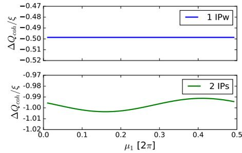
Figure 2: BB tune shift caused by single (1 IPw) and two head-on collisions (2 IPs) as a function of phase advance between the two collision points.
