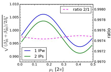
Figure 3: The combined beta-beating of two beams as a function of phase advance between two IPs, for a head-on collision, as measured at the scanning IP. Shown for a single collision at another IP (1 IPw) and including also the second collision (2 IPs)
