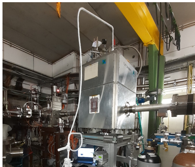
Figure 4: CCC cryostat during LN filling. The system is installed in an experimental cave at the SIS18 beamline.
