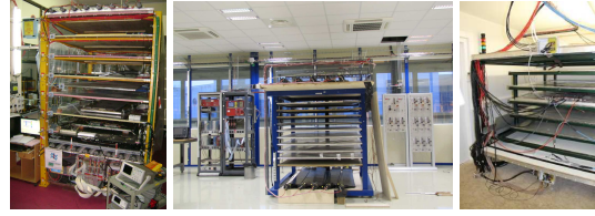
Fig. 9, Cosmic hodoscopes at RPC labs., at NPD-BARC, Mumbai (left), CERN-904 site (middle) and Ghent site (right)
