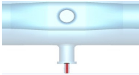
Figure 8: A modified design of electrically coupled antenna.
