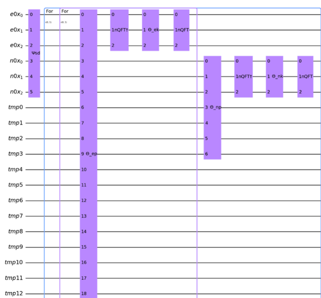
Figure 1. Circuit diagram of generated results for d = 1 , n = 3 , \eta = 1 , L_n = 1 , and N_E = 1 . The overall circuit consists of state-preparation and time-evolution gates. The initial state is prepared by the SD state preparation gate, \Psi_{sd} , and then, nested time evolution loops are applied to the state. The inner electron time-scale loop consists of an electron P.E. time evolution gate, \Theta_{ep} , an n -element inverse quantum Fourier transform gate, nQFT^\dagger , an electron K.E. time evolution gate, \Theta_{ek} , and an n -element quantum Fourier transform gate, nQFT . The outer nucleus time-scale loop consists of the inner loop, the nucleus P.E. time evolution gate, \Theta_{np} , the nQFT^\dagger gate, the nucleus K.E. time evolution gate, \Theta_{nk} , and the nQFT gate.
