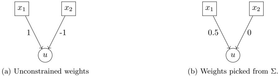
Figure 9.5: A neural network before (left) and after (right) the quantization with alphabet \Sigma = [-3, 0, 0.5] . Each weight is replaced with the closest one in \Sigma .
