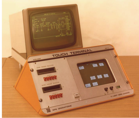
Fig. 5.10. The “Touch Terminal”, equipped with a CRT and driven by a 16-bit microprocessor.
