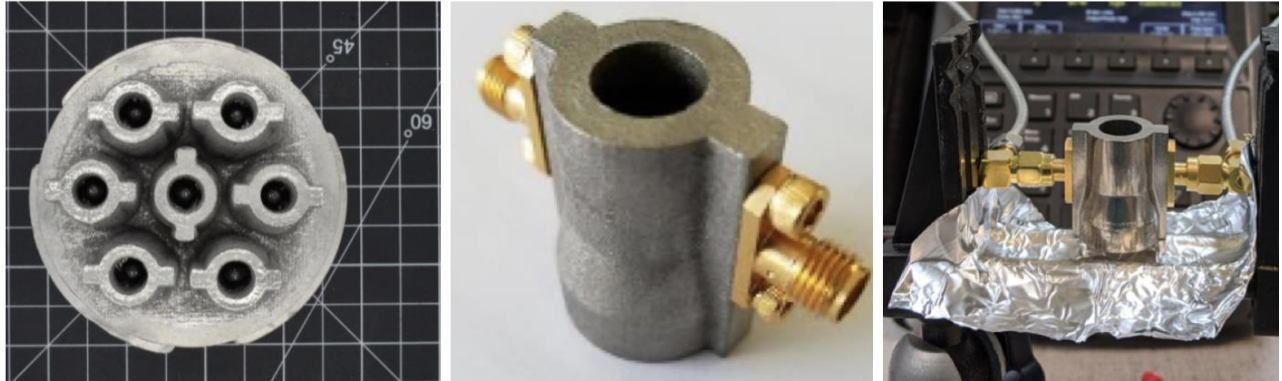
Figure 1: (Left) Array of niobium QWRs printed using EB-PBF on a titanium build plate; (Center) Ti-6Al-4V (Ti64) L-PBF QWR fitted with SMA coupling ports; (Right) Ti64 SLM QWR undergoing room temperature RF testing.
