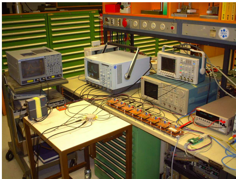
Figure D.3: Photograph of the experimental setup that was used to evaluate the performance of non-connectorized VCSELs.
