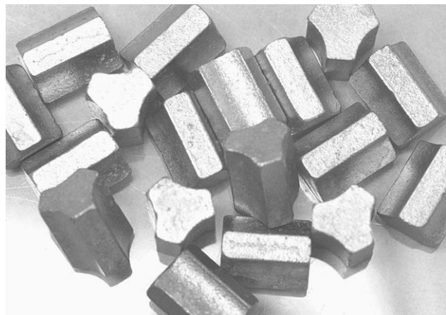
Figure 9-9 Sintered tungsten slugs as obtained for the engineering maquette.
