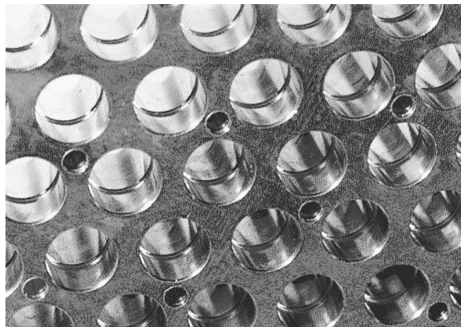
Figure 9-8 A close-up view of an end-plate, showing the grooves necessary for the swaging operation and the ground pin holes.
