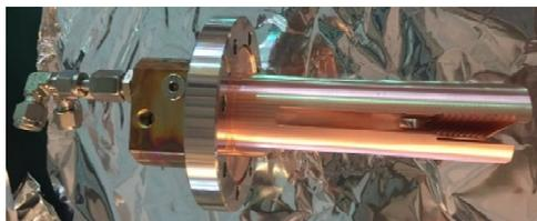
Figure 2: 2<sup>nd</sup> absorber without NEG coating.
