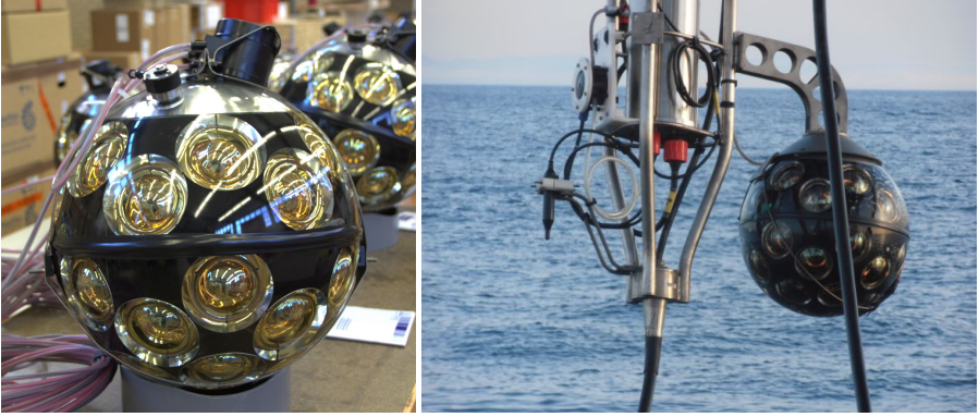
Figure 4.1: Left: A KM3NeT DOM with 31 small PMTs after assembly in the Nikhef workshop. The PMTs are arranged in horizontal rings of various zenith angles. Neighbouring PMTs within a ring are separated by 60^\circ , consecutive rings staggered by 30^\circ . Right: The PPM-DOM during deployment. It is connected on the first storey of the ANTARES Instrumentation Line. The metal structure is a standard ANTARES LCM which provides the DOM with power and data read-out.
