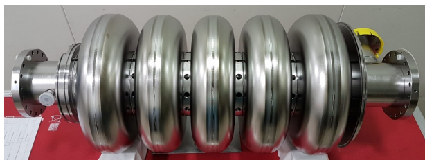
Figure 2: INFN B61_EZ_001 LB650 cavity for PIP-II.
