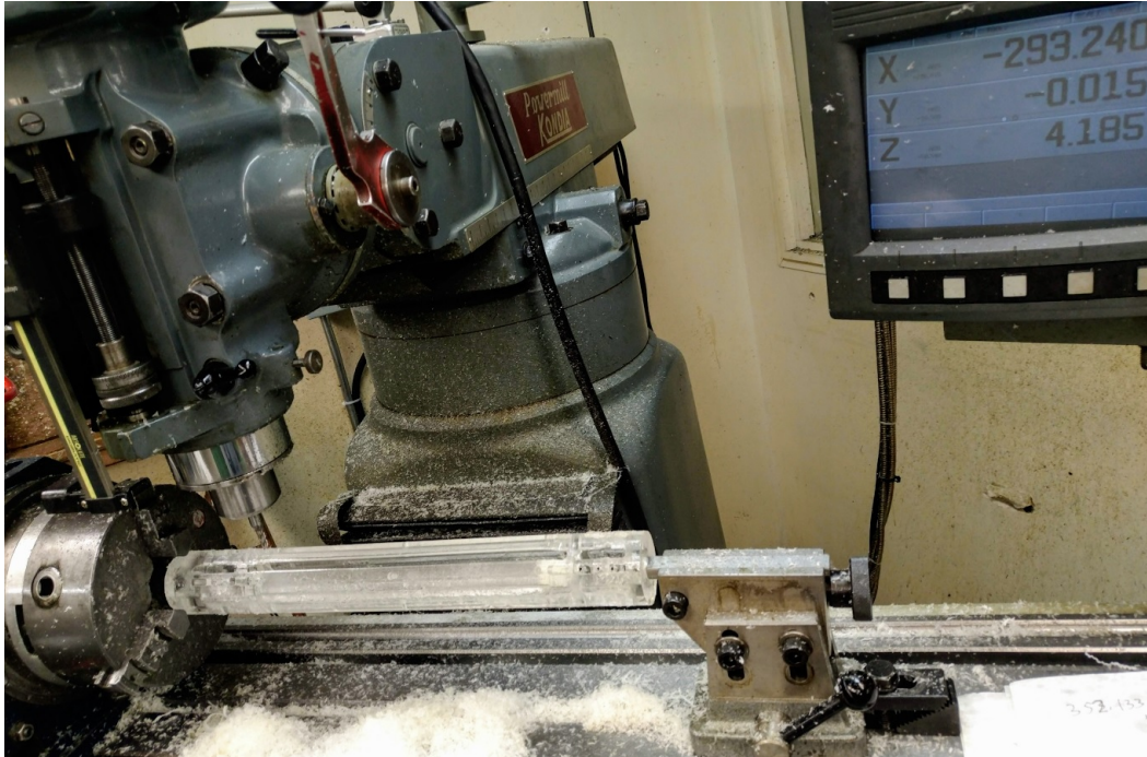
Figure A.1: Machining of the QMF1's monolithic holder.
