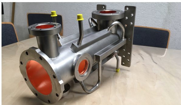
Figure 6: Quarter-wave resonator cavity prototype.
