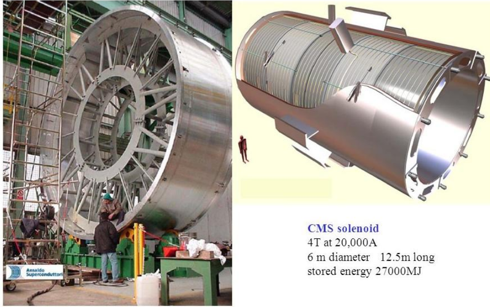
Figure 3.16: View of Superconducting magnet used in the CMS detector. Image source: https://images.slideplayer.com/36/10648021/slides/slide_21.jpg
