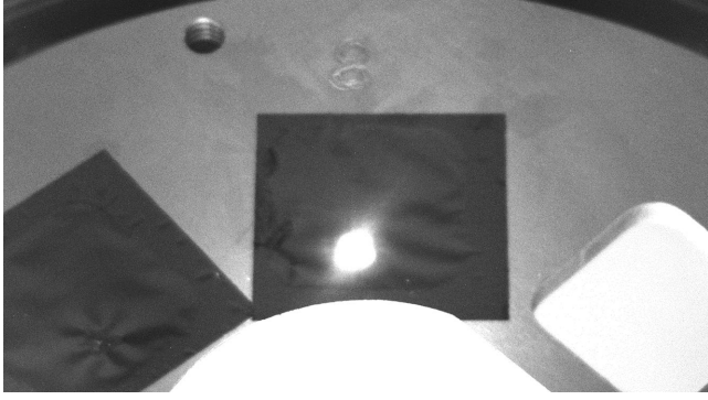
FIG. 9. cw argon beam image on carbon stripper foil. The beam rms and full diameters were 1 mm and \sim 3 mm, respectively.
