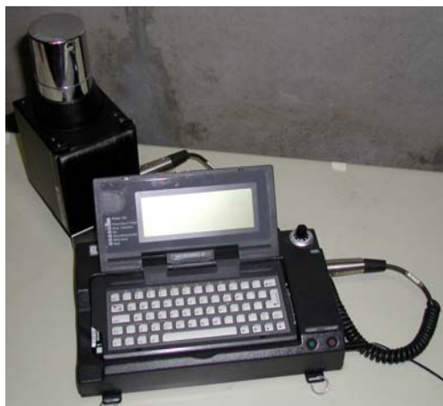
Figure 4. Instruments used to measure remanent dose rates: Microspec (left) and Eberline (right)
