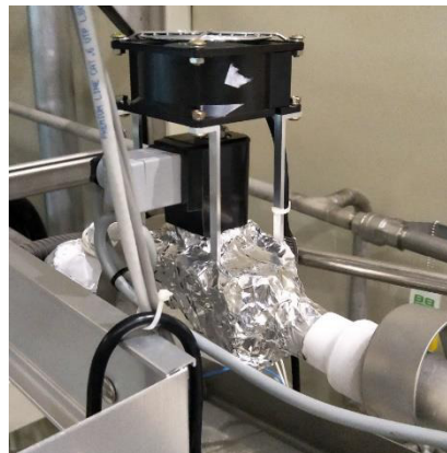
Figure 11: After install protection instrument, there is no condensed water or frost surround the relieve valve (foil covered) at LN 2 refilling period.
