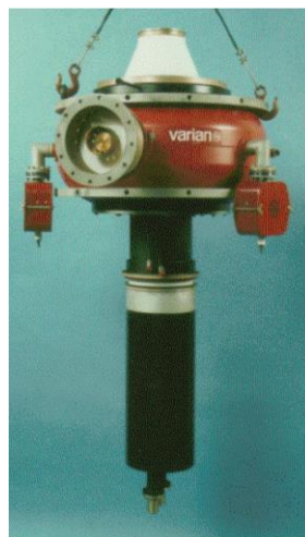
Figure 11: 250 kW CW, 267 MHz “Chalk River” IOT.
