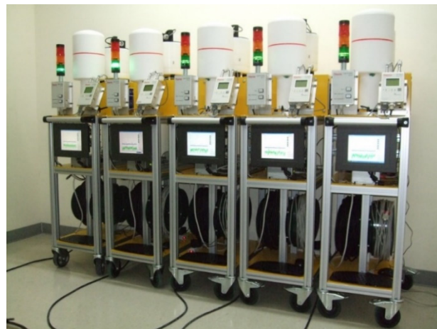
Figure 3: Real-time radiation monitoring stations with interlock.
