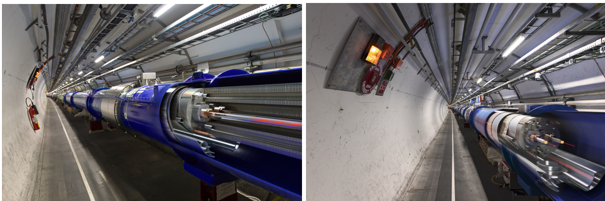
Figure 2-2. 3D-rendered cut-out section of a LHC superconducting dipole magnet [8].
