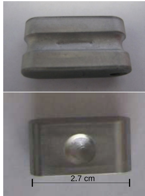
Figure 1: A slit cathode (top) and a dimpled cathode (bottom).
