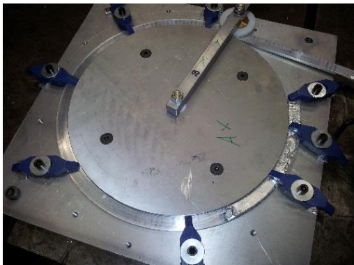
Fig. 7: DS2 cable during the hard-way bending process at INFN Genoa .
