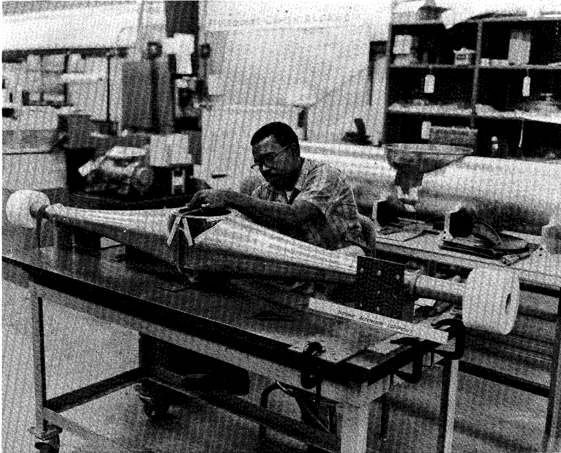
Fig. 9. Clinton Martin assembling the drift-tube section of a prototype booster cavity.
