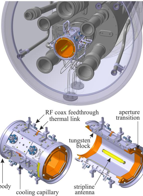
Figure 2: BPMQSTZB-type cryogenic directional coupler BPM in a magnet's cryostat (top) with its most important features marked (bottom).
