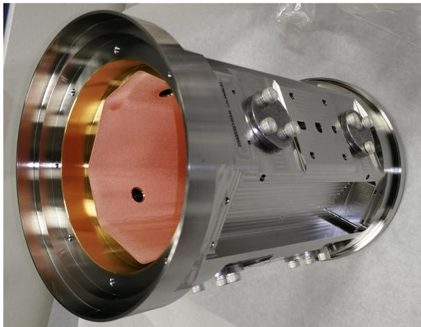
Figure 3: Gold- and copper-coated pre-series body of the BPMQSZTB-type BPM
