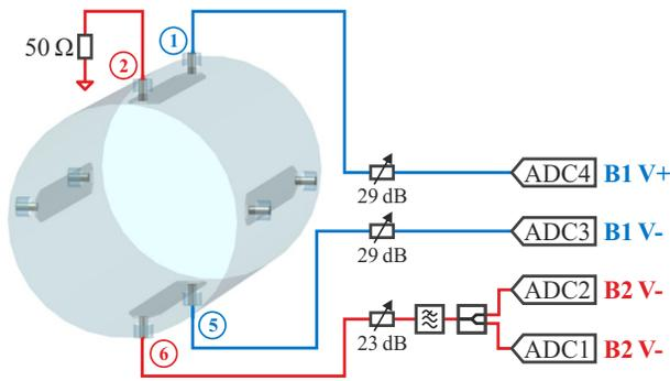
Figure 4: One of the configurations used in 2021 to acquire beam-induced BPM signals with a ZCU111 board.
