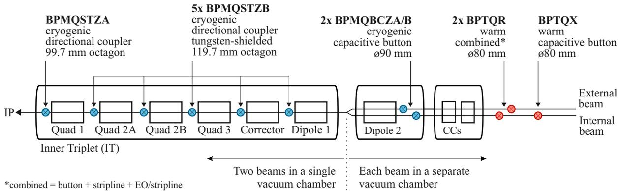
Figure 1: New BPMs foreseen to be installed in the HL-LHC era on each side of the ATLAS and CMS experiments.
