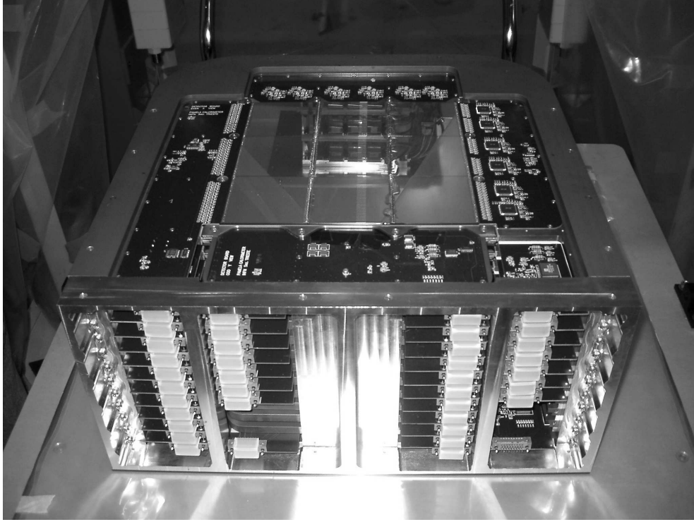
Figure 1.23: the imaging calorimeter of PAMELA; the first silicon plane and its support board housing the corresponding FE electronics are visible on the top.
