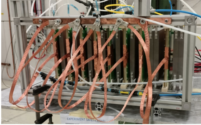
Fig. 4.11: Left: MPGD-based HCAL prototype tested at CERN having multiple layers built with different technologies. Right: measured MIP-detection efficiency of different MicroMegas layers as a function of the applied high voltage.
