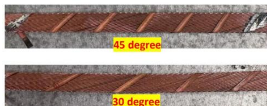
Figure 1: REBCO wrapped Rutherford type cables
