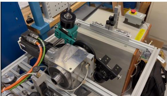
Figure 3: 3D-printed assemblies mounted to motor hub
