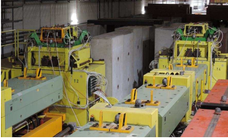
FIGURE 6.5: LEFT: Primary targets T2 and T4. Along with a set of targets, the station contains beam monitors for positioning of the beam on the target, intensity measurements etc. RIGHT: Split-foil beam monitors: two sets of top-bottom and left-right imbalance monitors provide the data for target centering.
