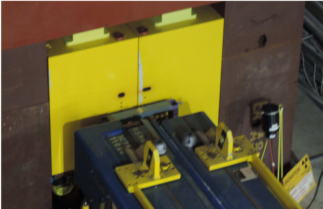
FIGURE 6.8: TAX blocks of the beam lines H2 (right) and H4 (left). The movable TAX blocks provide a selection of collimators and serve as a first stage of the secondary beam momentum selection.
