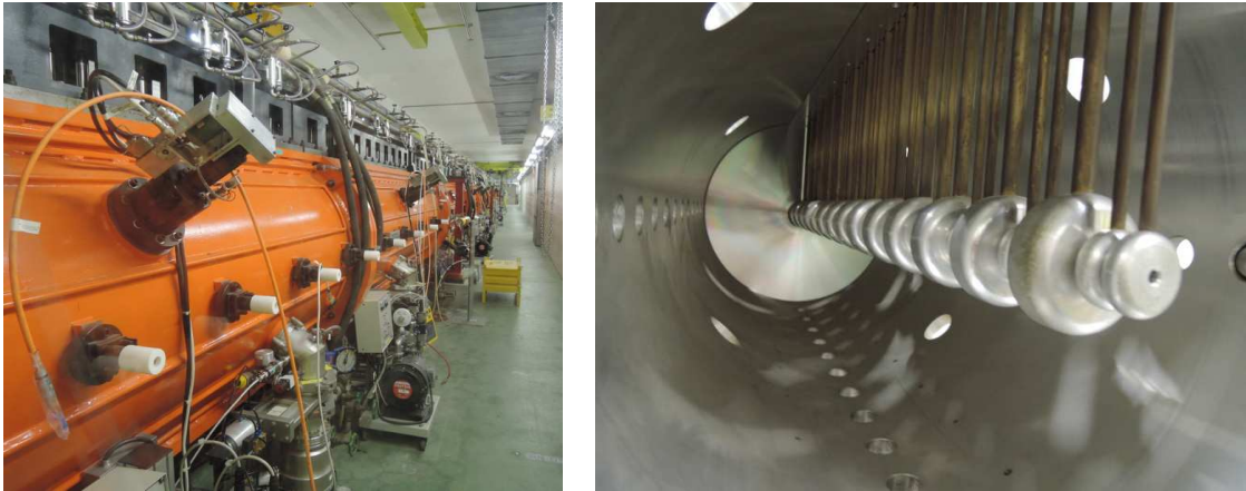
FIGURE 3.4: Linac2. LEFT: Array of Linac2 tanks. RIGHT: Drift tubes inside of the Linac2 tank. The picture is taken through the service opening of the vacuum vessel displayed in the Linac2 complex.
