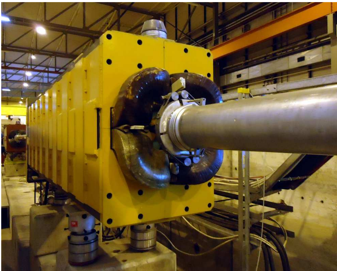
FIGURE 6.12: One of the Quadrupole magnets in the H2 beam line. Most frequently used for focusing of the beam on the main experiment, if needed, they can also be used to create quite sophisticated beam profiles.
