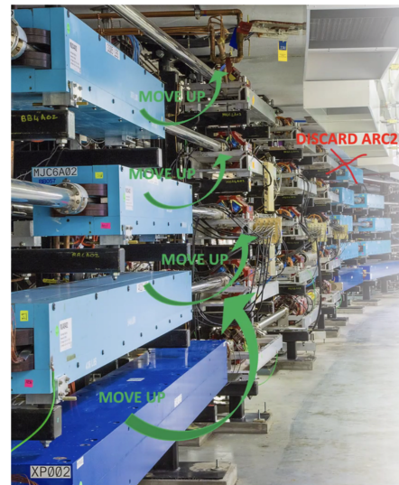
Figure 3: Image showing the “promotion” of the magnets and optics from the higher energy passes to the lower energy passes.
