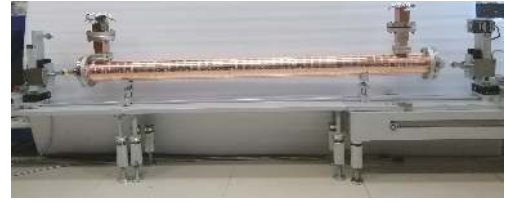
Fig. 5 Hybrid bunching-accelerating structure prototype after welding
