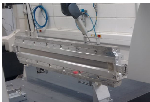
Figure 6: CMM measuring process.
