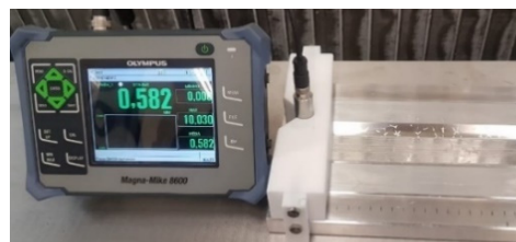
Figure 5: Prototype under measurement with the Magna Mike 8600.
