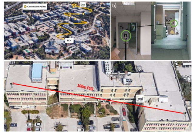
FIGURE 2 (a) Installed intra-campus 2.2-km fibre link, (b) 40-m indoor FSO link, (c) Map of 100-m FSO link interconnecting two ECE building's rooftops [©2024 Google]. ECE, Electrical and Computer Engineering; FSO, Free-Space Optical; IC, Intra-Campus.
