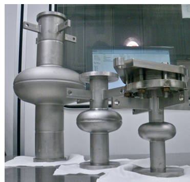
Figure 1: Left to right: A 1.3 GHz, 2.6 GHz, and 3.9 GHz Nb 3 Sn cavities. The 3.9 GHz cavity has a top plate and clamps attached for testing.
