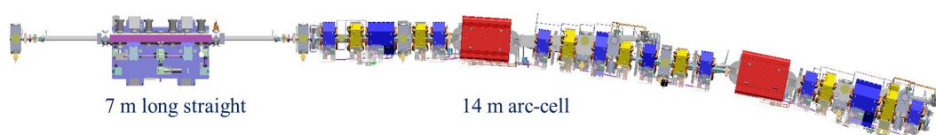
Figure 1. Assembly drawing for a typical sextant super-period vacuum system with magnets.
