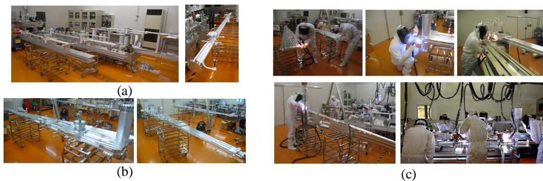
Figure 5. Photographs of (a) welded S-chambers, (b) welded B-chambers, and (c) welding works for the B-chamber.
