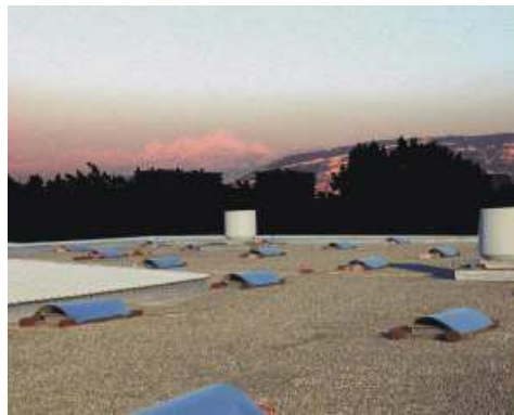
Figure 18: The air shower scintillator array on the roof of the surface hall ( 54 \times 30 \text{ m}^2 ) and the L3 detector covered with timing scintillators in the LEP cave.)
