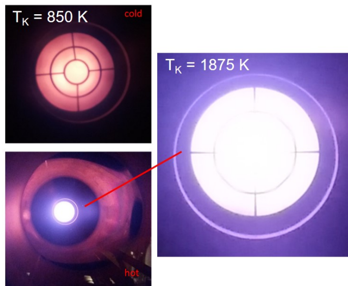
Figure 5. An example of cathode heat-up measurement and proof of principle, measured temperature given at emissivity factor \varepsilon = 1 .
