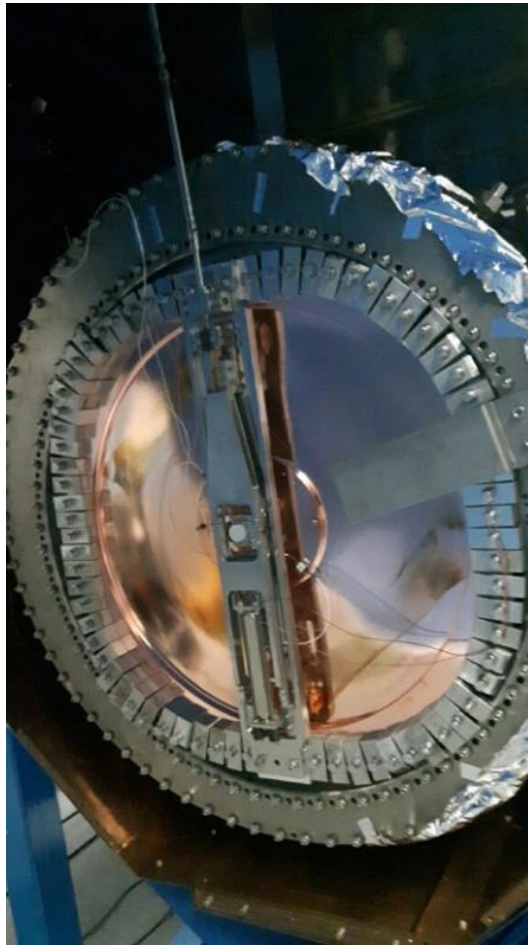
Figure 3: Photo of the combined slow+fast tuner, assembled onto one SRFQ end-plate
