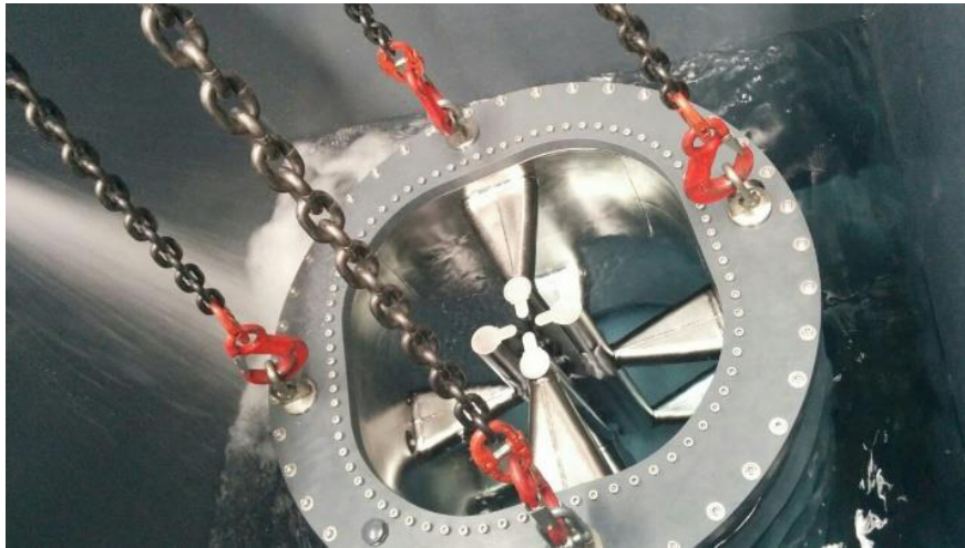
Figure 1: SRFQs during BCP at CERN.
