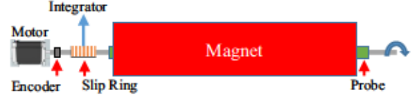
Fig. 3. Principles of a rotating coil system.
