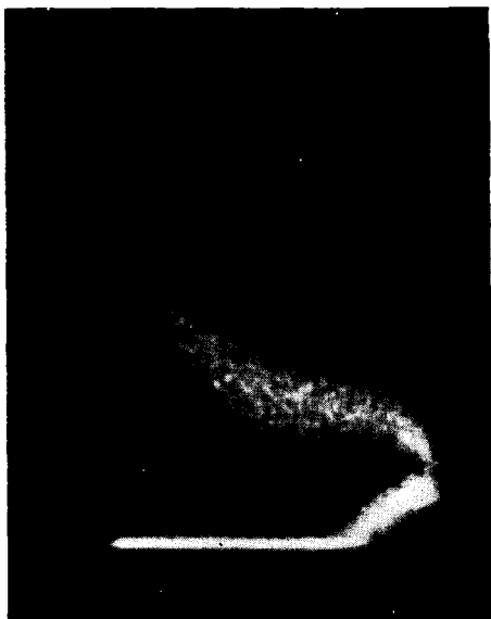
Figure 9 Separation of neutron and gamma ray pulses in p-terphenyl-POPOP-toluene phosphor using space charge saturation in RCA 6810.
