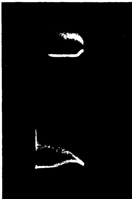
Figure 8 Separation of neutron and gamma-ray pulses in stilbene using space charge saturation in EMI 6097.
