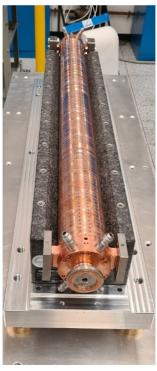
Figure 7: Insertion of the assembled structure in the vacuum furnace for brazing and brazed final prototype.
