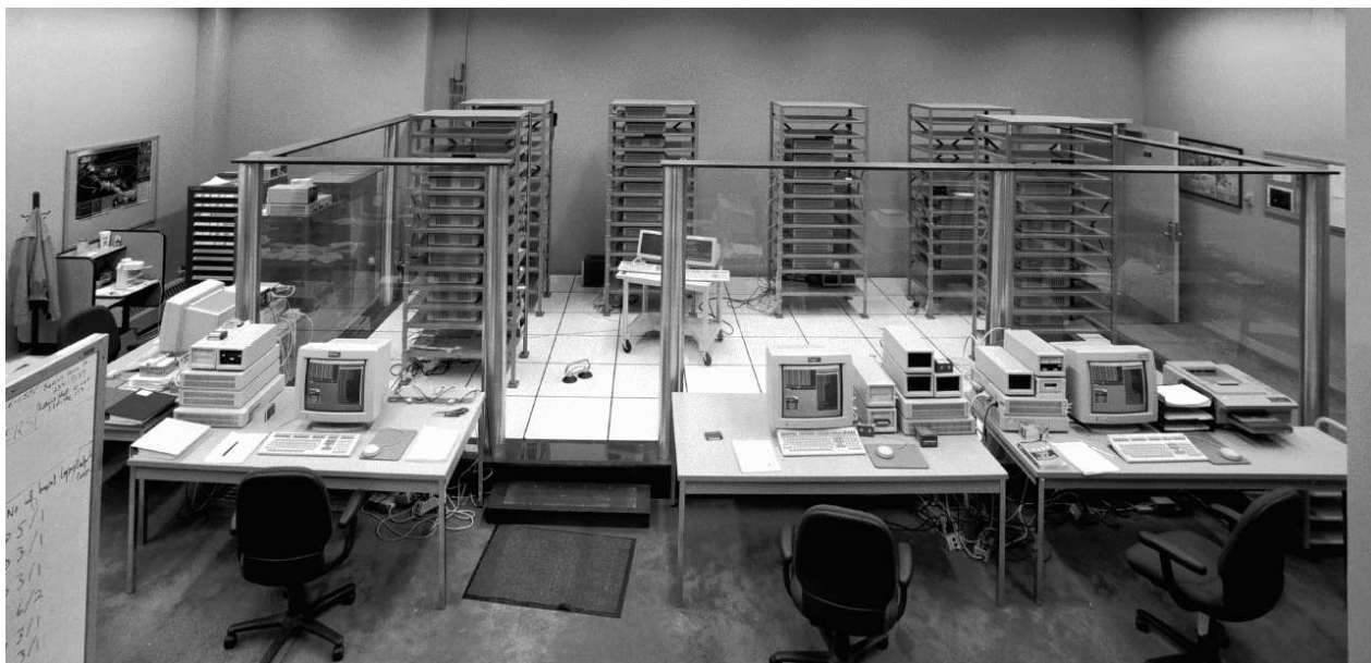
Fig. 2. A photographic overview of the University of Mississippi computing farm. Servers are on the four tables. Clients are on the racks shown and on desktops which are not shown. If the room overheats, power is automatically cut to the computers and must be manually reset. The espresso machine is on the left.
