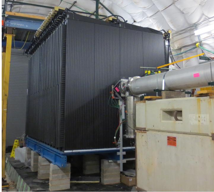
Figure 3.9: Picture of the NOvA Test Beam detector in the MC7b enclosure at the Fermilab Test Beam Facility. The silver tube to the right (upstream) of the detector is the Cherenkov detector.
