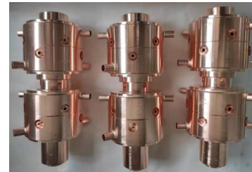
Figure 4: Photo of brazed correction cavity pairs.
