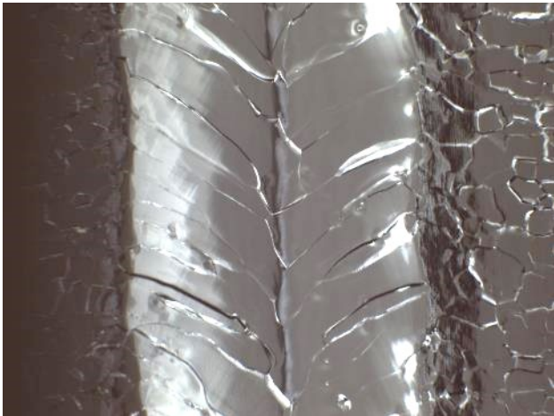
Figure 4: Photo of inner surface at one equator of FG #3 cavity, which shows no defects.
