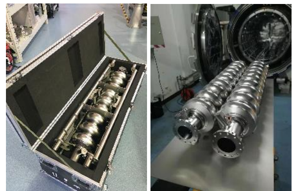
Figure 2: First FG cavity fabricated by Group-1 in the shipping box and two LG cavities fabricated by Group-2 after 750°C annealing.
