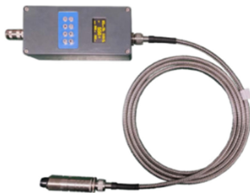
Figure 5. A physical picture of the colorimetric thermometer.
