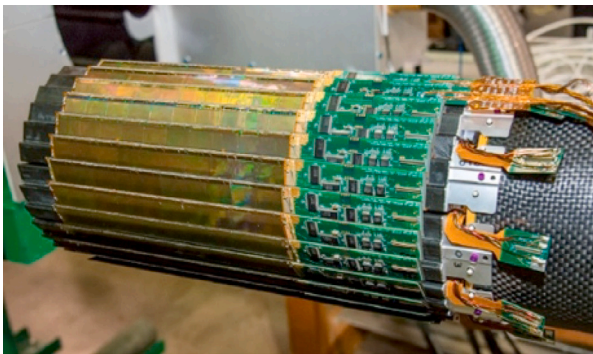
Fig. 7. Photograph of the vertex detector of the STAR experiment [58], the first to use CMOS MAPS.
